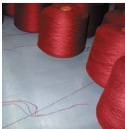
Transportband aus Polyester-gewebe, Masche 1X1 mm für Hochfrequenz-trockner. | Conveyor belt made of Polyester Fabric, mesh 1X1 mm for high frequency dryers.
